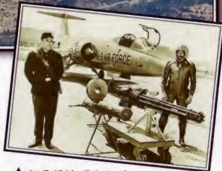
▲ An F-104A pilot stands next to the powerful 20-mm (0.79-in) Vulcan cannon fitted to the USAF Starfighters and one of its ancestors, the nineteenth-century Gatling gun.
